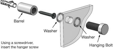
Using a screwdriver, insert the hanger screw through the barrel and into the nylon anchors, then tighten to surface.
